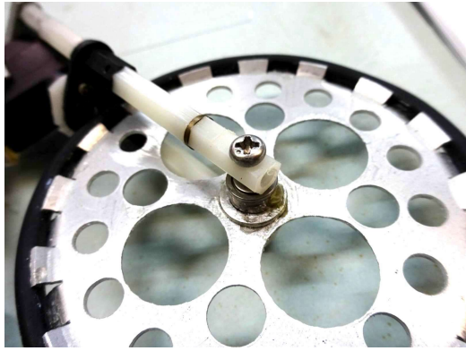
Photo 7.14 Example of making a wheel from aluminum plate
